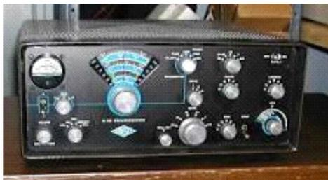
not a true transceiver, in that it does not transmit and receive on the same frequency unless the operator puts the internal VFO on the same frequency manually. The internal VFO does not work on six meters; six operation is only crystal controlled transmission. Except for six meter coverage, the G-76 is essentially a G66 receiver and G-77 transmitter in a single box. The concept of putting a
